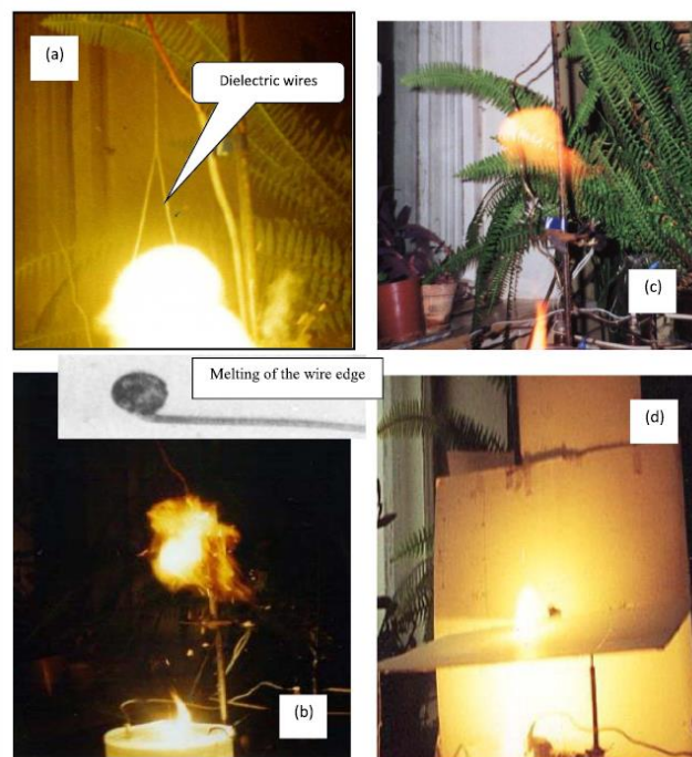
Figure 12. Additional evidence of the close relationship between the observed plasmoids and natural BL. Absence of interaction with dielectrics (a); strong interaction with conductors (b); good transparency (c); penetration through a hole displaced from the discharge axis by 3 cm and smaller than the diameter of the plasmoid (d).
